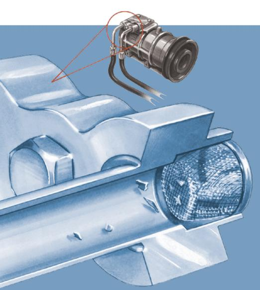
magine this, you've got an Air Con Machine which needs servicing, it works perfectly for a few months and then it packs up again, why? Compressor Guards. These vital little guardians protect you and your machine's warranty by stopping any debris from entering the compressor.
